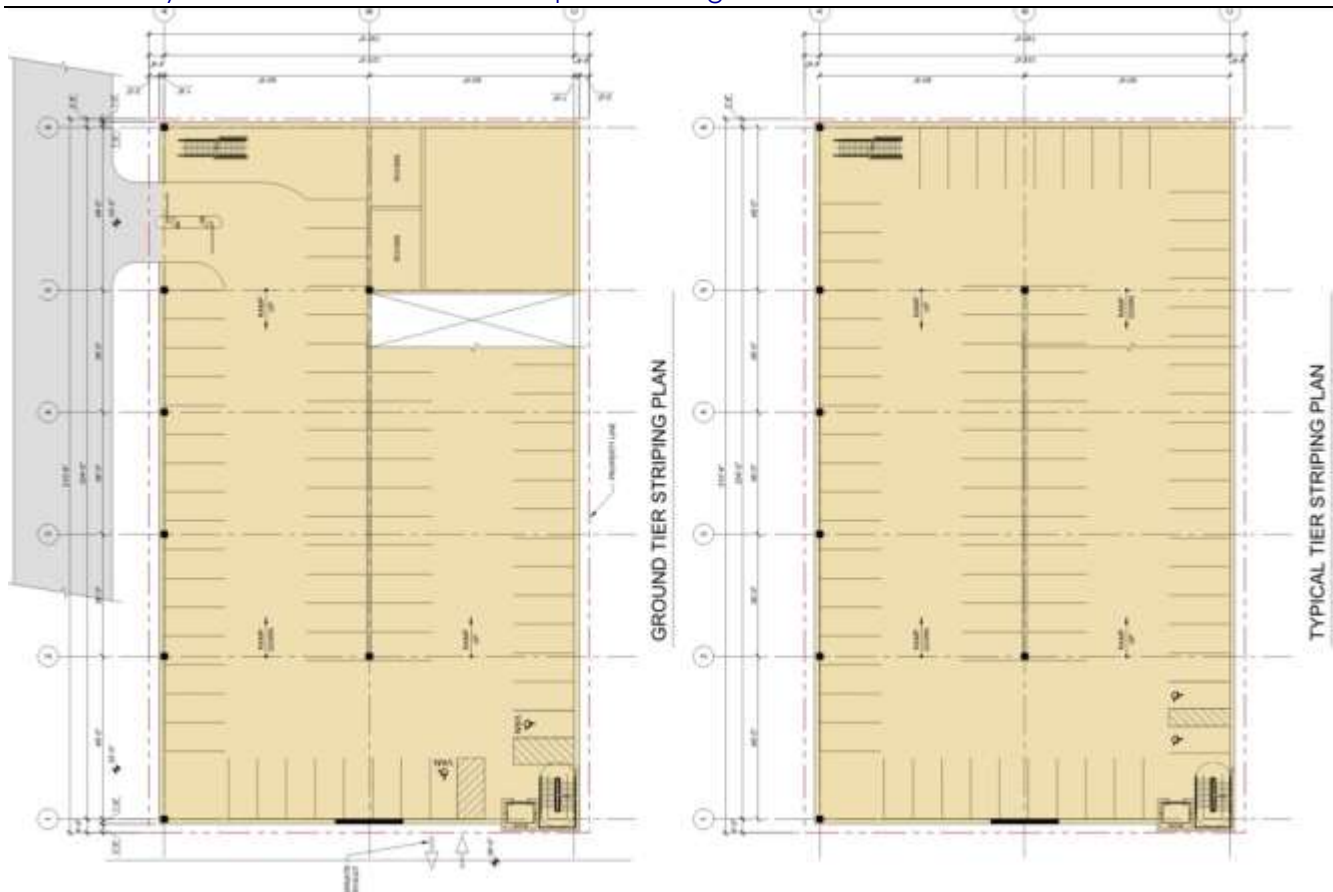
Exhibit 8: Layout and Function of a Conceptual Parking Structure
