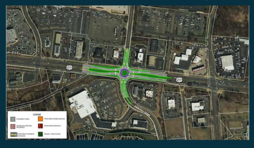
General Concept is to install a roundabout to keep circulation moving with the other roundabouts and improve safety. Final Design to be determined.
