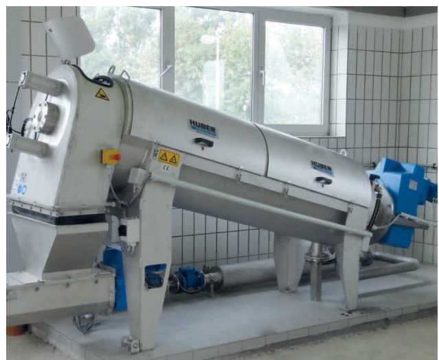
Stationary mounted screw press for 140 kgDS/h
