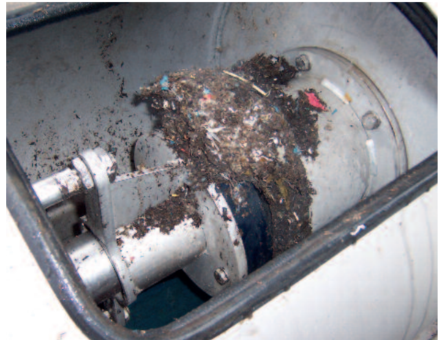
Discharge of the separated dewatered material
