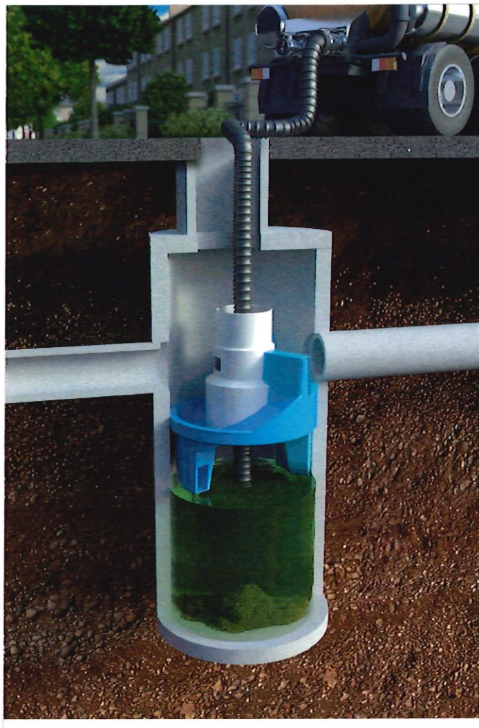
Fig.4 Floatables are removed with a vector hose
