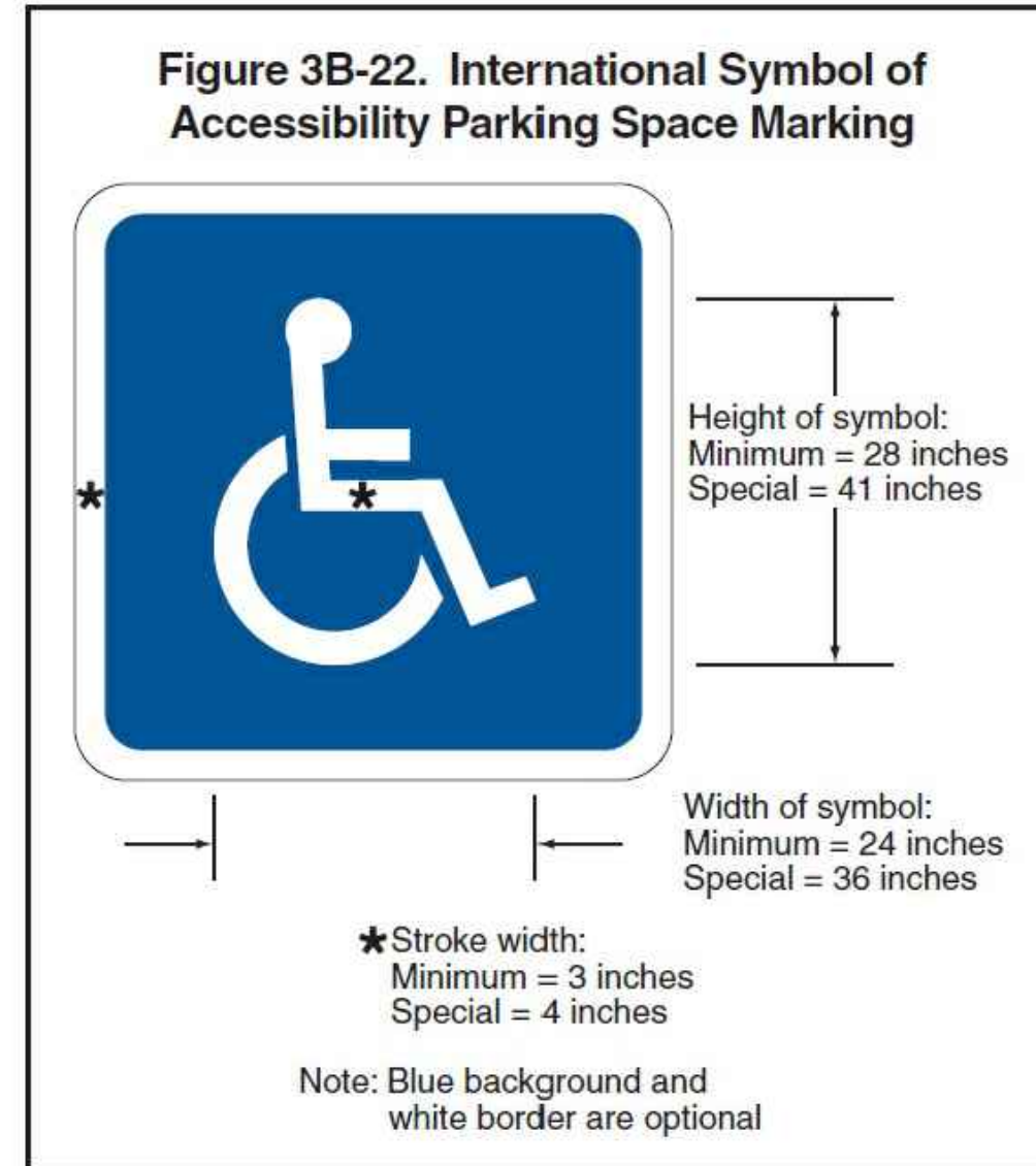
HANDICAP PAVEMENT MARKING DETAIL SCALE: N.T.S.
