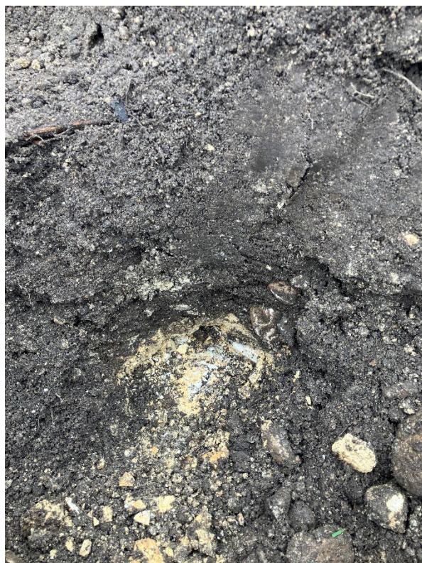
Photograph 3: General view of DP-1U soil pit and rock encountered at 18 inches below ground surface.
