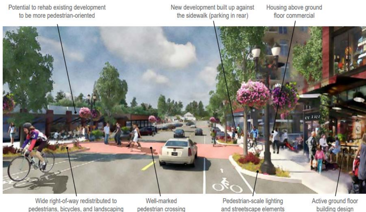
Figure 5. Rendering of a Cleveland Avenue streetscape after a road diet (Brewery District Plan)
