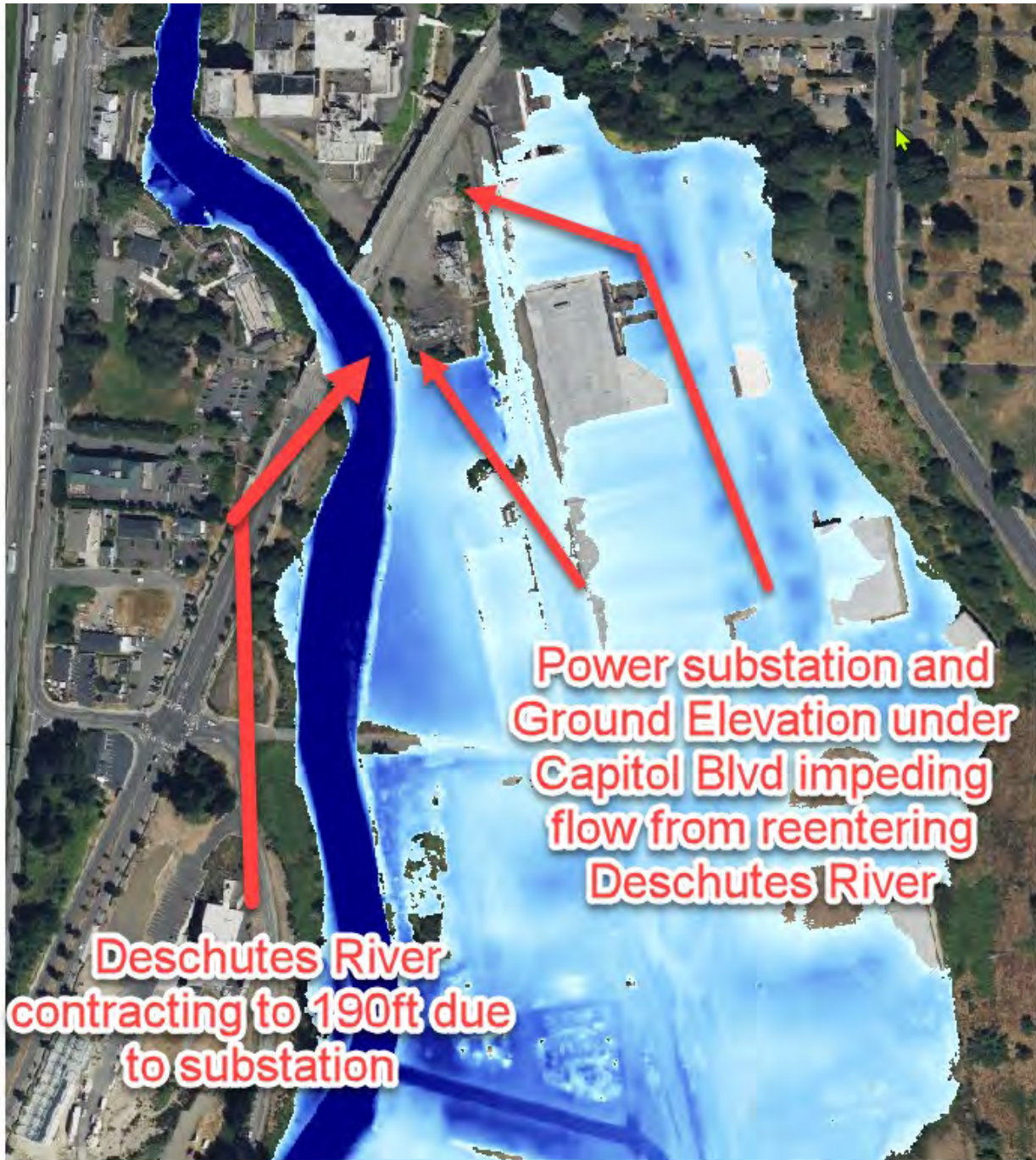
Figure 25 – Illustration of Power Substation and Ground Under Capitol Blvd Impeding Flow
