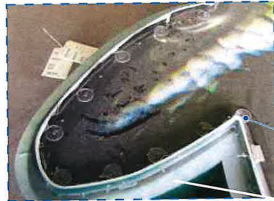
Tail section only, attached with polycarbonate (Lexan) wafers along fish tail section.
