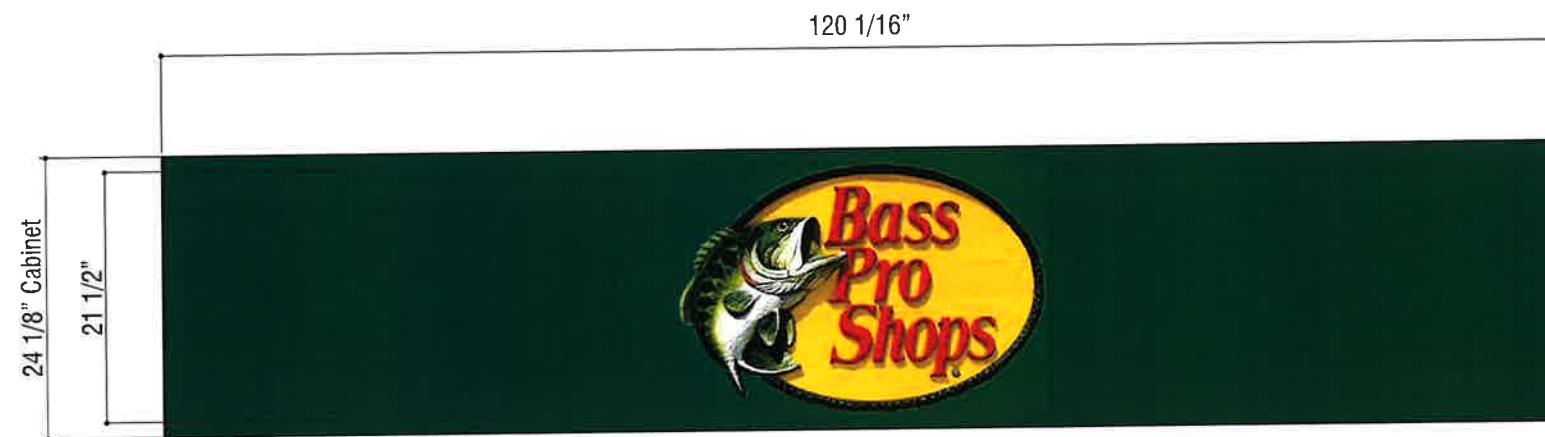
1 D/F Illuminated Pylon Sign Reface 20.1 sf Scale: 3/4" = 1'-0" (2) Faces Req'd.
