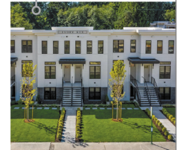
DON'T Allowing a higher front setback (10 feet or greater) for residential uses that do not have vehicle areas in the front façade is not compatible in placetypes promoting the highest level of pedestrian activity. Buildings with a setback greater than 10 feet tend to lose the relationship between the sidewalk and the building.
