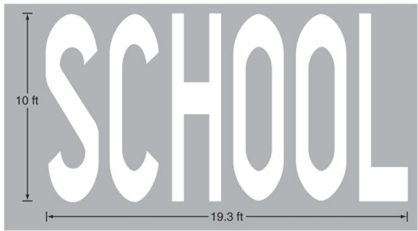
Figure 7C-1. Two-Lane Pavement Marking of "SCHOOL"
