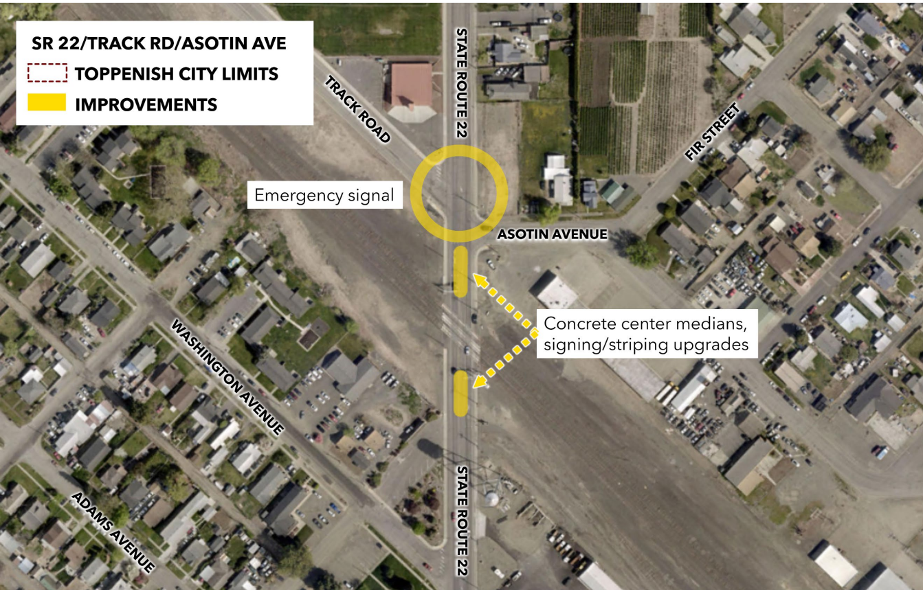
FIGURE 9: STATE ROUTE 22/TRACK ROAD/ASOTIN AVENUE IMPROVEMENTS
