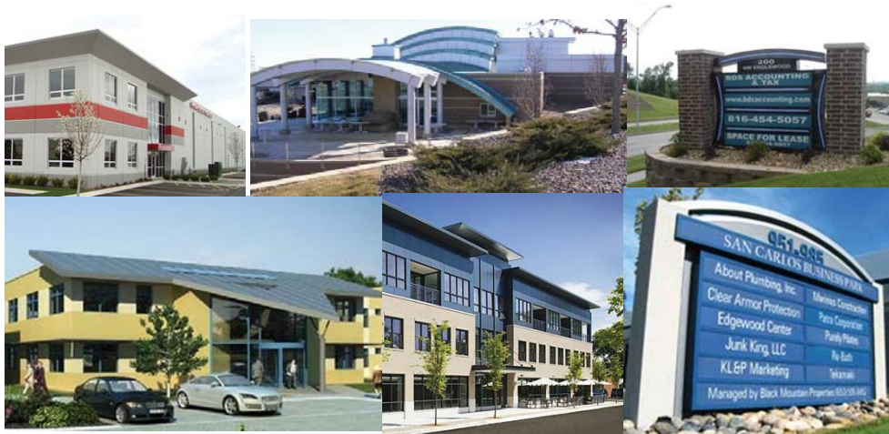
There are many ways to architecturally define building entrances on office/industrial buildings. Figure 3.6 demonstrates a few examples with a varying degree of protection provided, along with examples of common directory signs at business/industrial park entrances.
