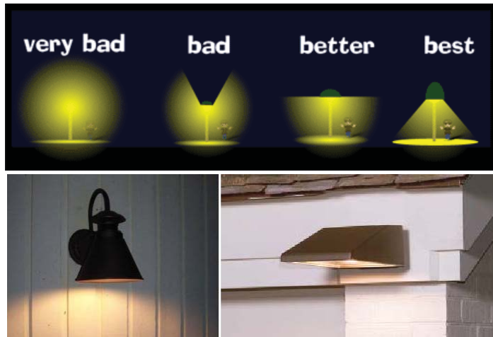
Figure 3.9 illustrates the different types of lighting techniques from no cutoff to full-cutoff. The lower images provide good examples of full-cutoff building light fixtures.
