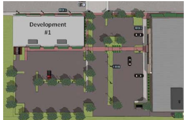
Figure 3.5 illustrates shared parking between two developments connected by an access drive, and includes vegetative buffers along all pedestrian routes.
