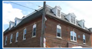
MANSARD ROOF (with dormers)
