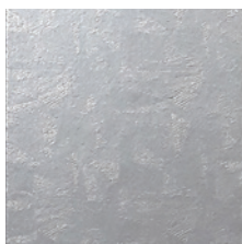
Acrylic Coated Galvalume TSR = 55%
