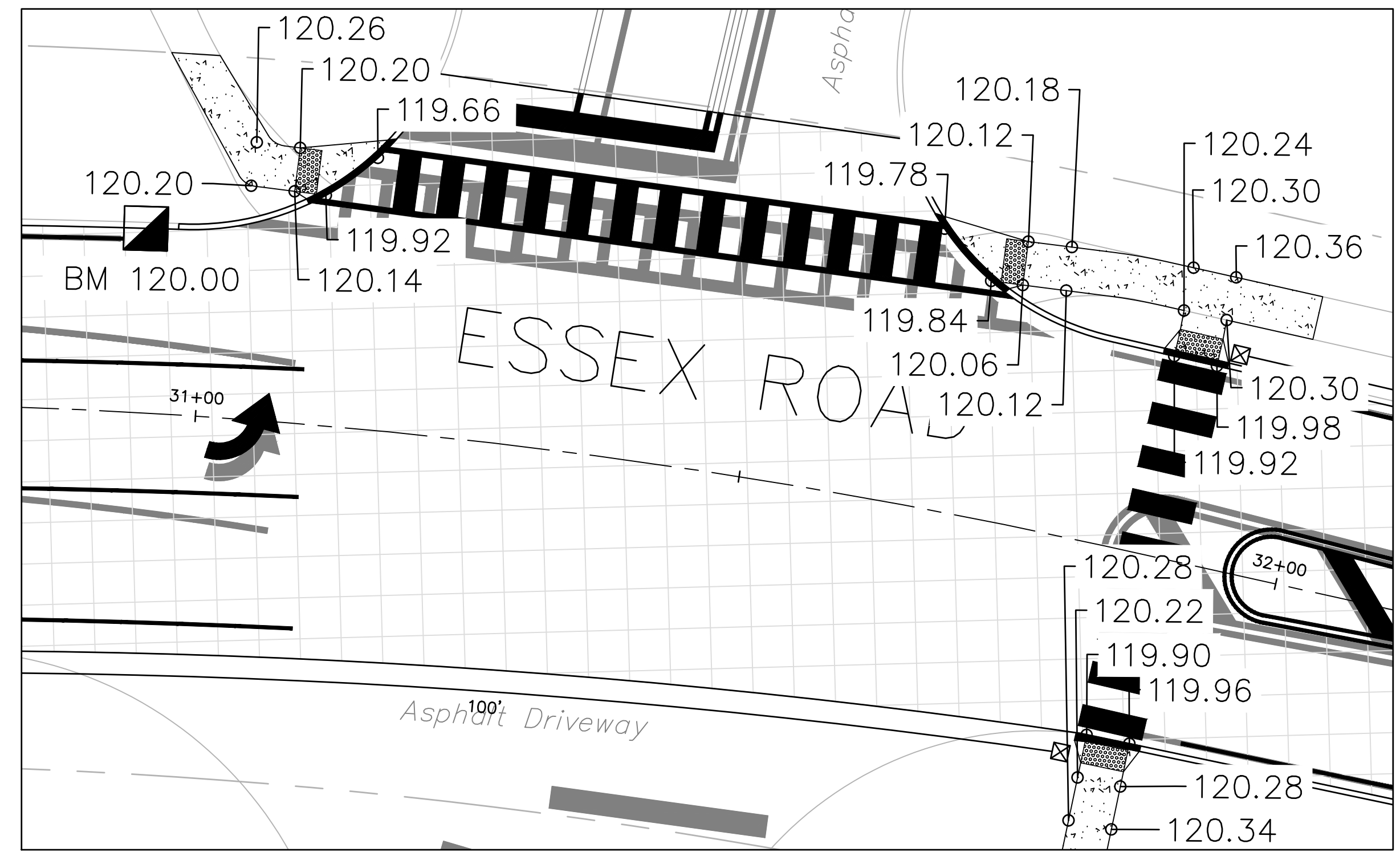
CURB RAMP GRADING PLAN ESSEX ROAD & JERSEY SHORE OUTLETS ENTRANCE SCALE: 1" = 10'
