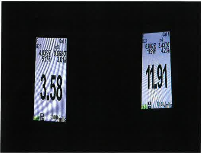
PRIMER DFT LOW AND HIGH READINGS
