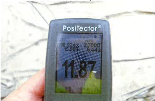
DFT READINGS, LOW/HIGH/AVG
