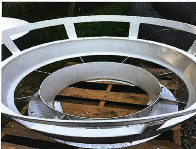
FROST FREE ROOF VENT COATED
