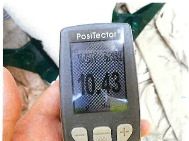
INTERMEDIATE COATING DFT READING
