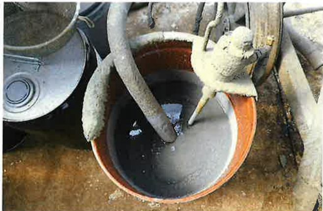
AIR AGITATOR FOR PAINT MIXING
