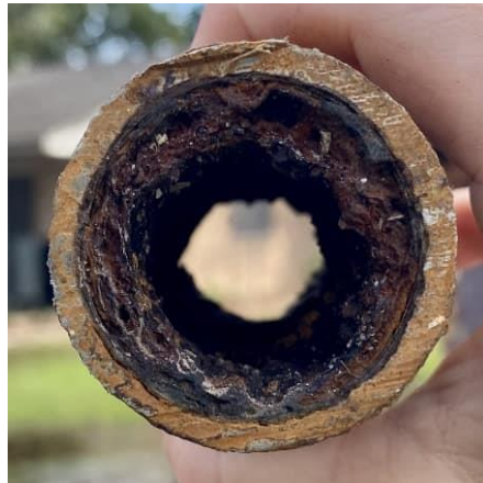
Section removed from Pecan St. waterline when staff repaired a major leak at Pecan & 4 th St. in August 2023.
