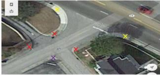
X = Remove and replace existing with Type 1 directional curb ramp.
