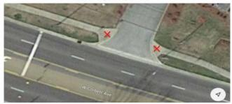
X = Remove and replace existing with Type 1 directional curb ramp.
