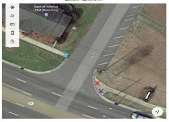
X = Remove and replace existing with Type 1 directional curb ramp. X = Remove existing curb ramp. X = Install raised truncated dome. (4 feet wide)
