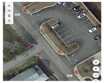
X = Remove and replace existing with Type 1 directional curb ramp.
