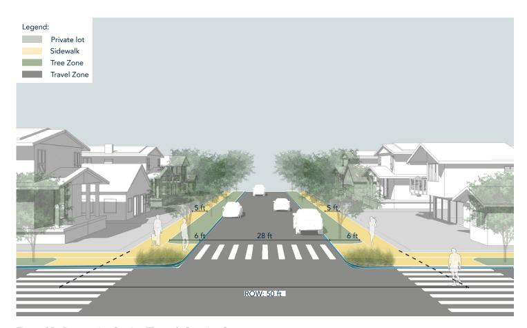
Figure 85: Perspective Section Through Queuing Street
