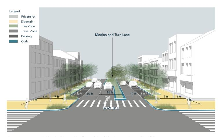
Figure 89: Perspective Section Through Collector Mixed-Use Street (New or Retrofit)
