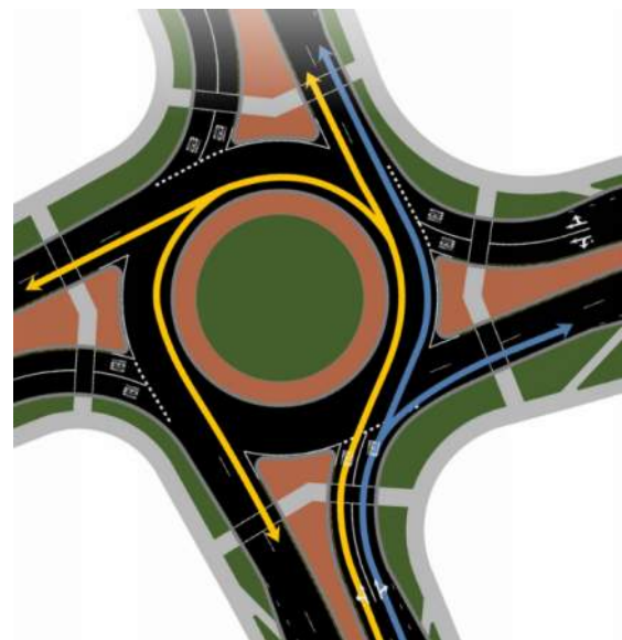
Illustrative roundabout showing traffic flow lines
