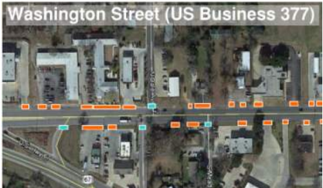
Excessive driveway access on busy arterial.
