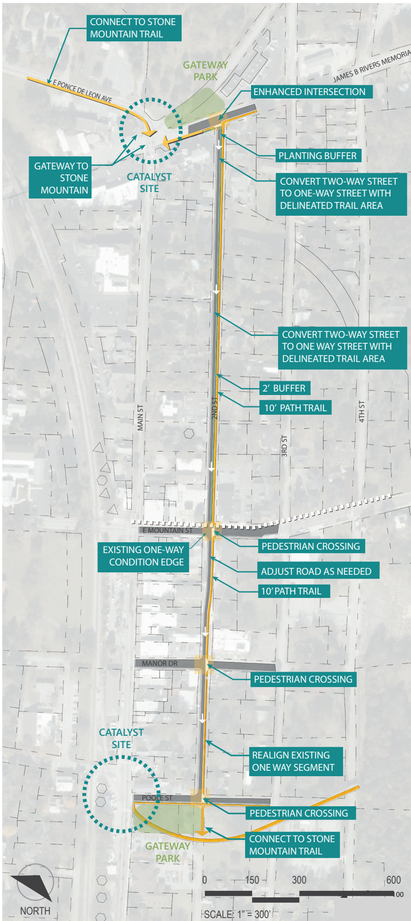
Figure 14: Second Street Alignment Recommendation
