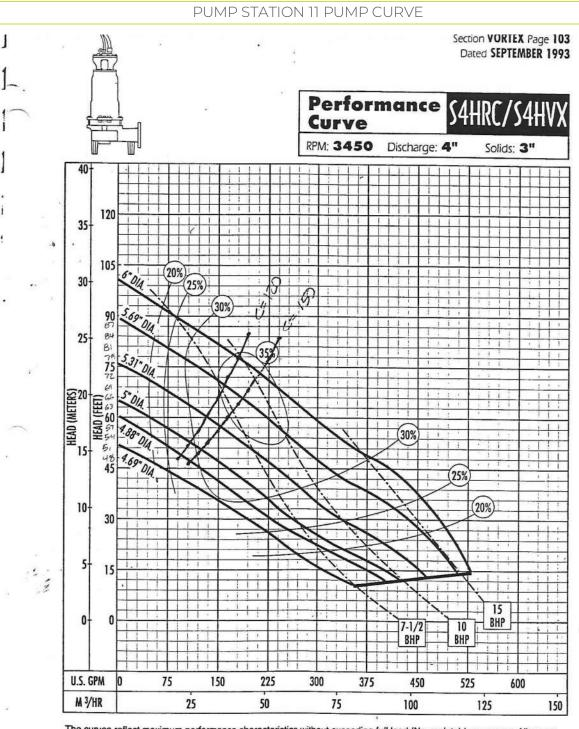
The curves reflect maximum performance characteristics without exceeding full load (Nameplate) horsepower. All pumps have a service factor of 1.2. Operation is recommended in the bounded area with operational point within the curve limit. Performance curves are based on actual tests with clear water at 70° F. and 1280 feet site elevation.
