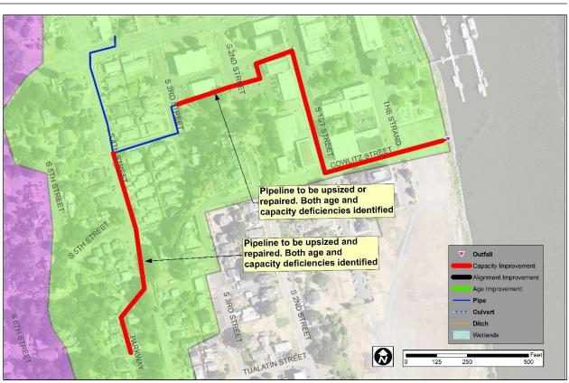
The two alternatives evaluated in this basin are targeted toward alleviating flooding in the pipe network along S 4th Street, which was identified through modeling, and to address the aged 24-inch pipes draining east to the outfall. The two alternatives considered are illustrated in Figure 6-7 and the improvement descriptions are provided below. Both alternatives include upsizing the pipe along Parkway as shown in Figure 6-7.
