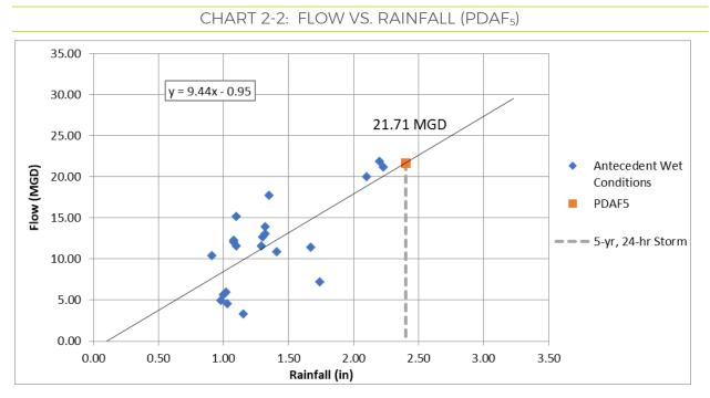
In analyzing the data, peak flows at the WWTP occurred on the same day or the following day as storm events. The PDAF<sub>5</sub> developed, using DEQ's method, was compared with the top five peak day flow events from 2015-2019 with antecedent wet conditions (see Table 2-4 below). The PDAF<sub>5</sub> observed in 2019 was selected as the planning value for this study because it is higher than the PDAF<sub>5</sub> flow developed using DEQ's method and is a more conservative planning value.
