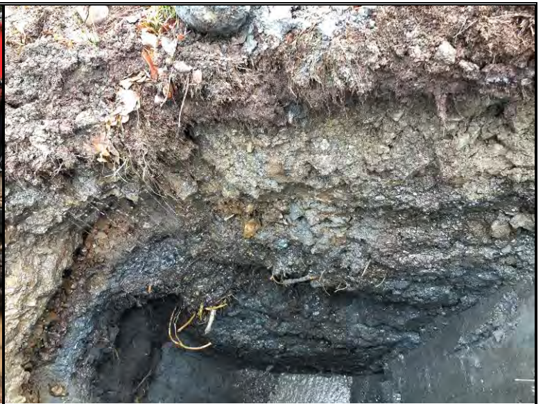
Exposed subsurface soil profile within test-pit TP-1
