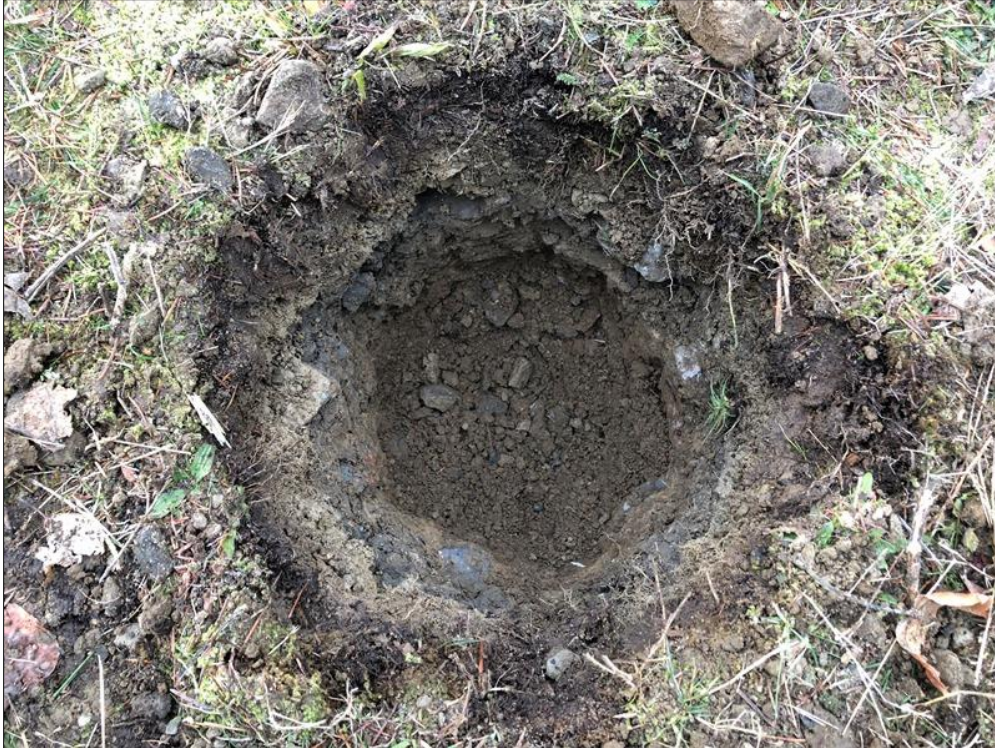
Figure 11. Representative view of the gravelly fill encountered in the STPs.
