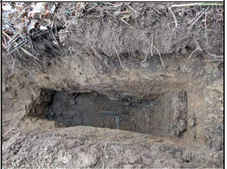
Exposed subsurface soil profile within test-pit TP-2
