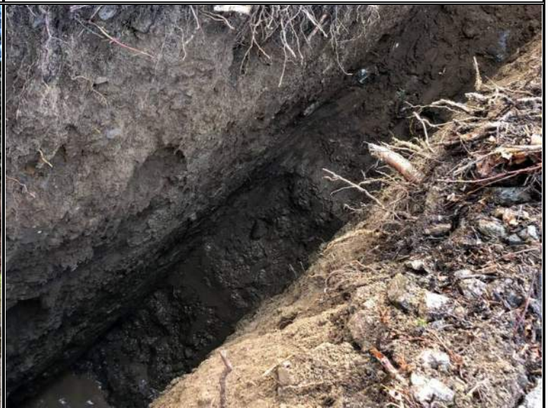
Exposed subsurface soil profile within test-pit TP-8
