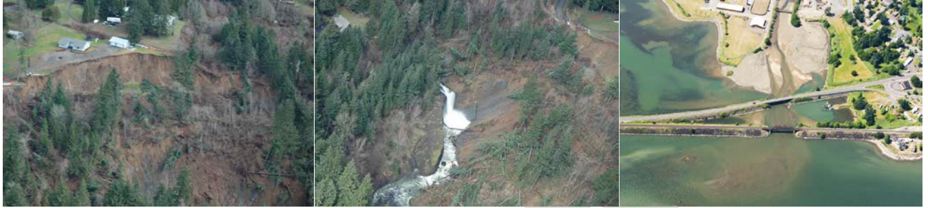
Rock Creek Reach 2 Degradation & Restoration Opportunities Scarp of Piper Road Landslide at Rock Creek's First Falls & resulting aggradation in Lower Rock Creek.
