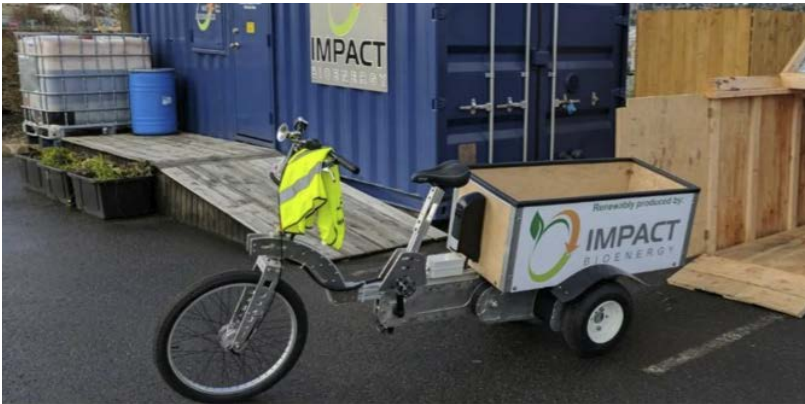
Figure 5 This electric cargo bike used for waste food diversion program runs 1 mile per pound of food waste according to Impact Bioenergy.
