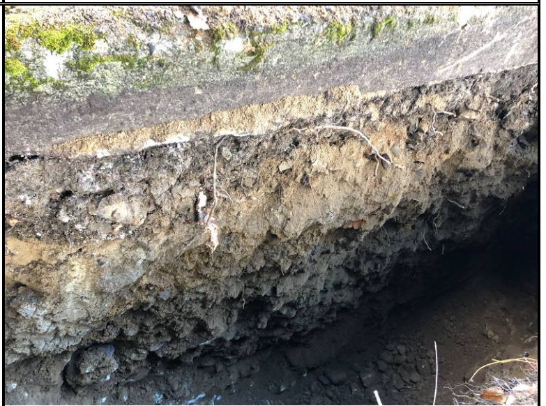
Exposed subsurface soil profile within test-pit TP-6
