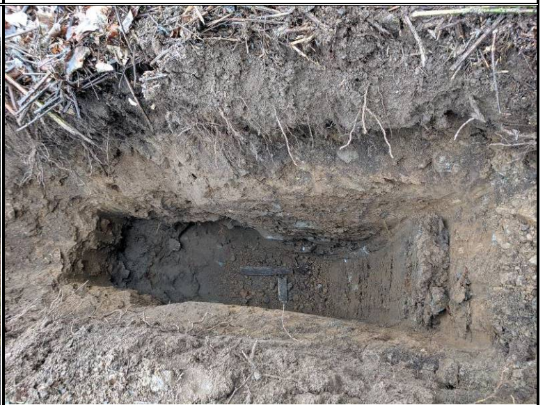
Exposed subsurface soil profile within test-pit TP-2
