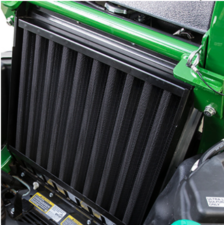
Radiator debris screen
