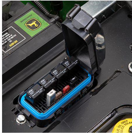
Sealed fuse and relay box
