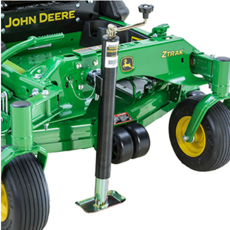
Jack kit and jack installed
