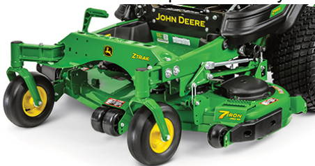
54-in. (137-cm) 7-Iron PRO Mower Deck
