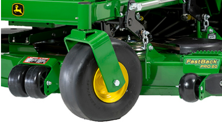
Center deck rollers and left wheel
