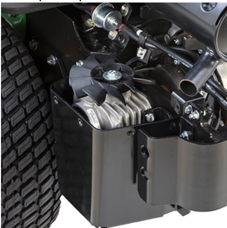
Right angle gearbox with cooling fins and fan
