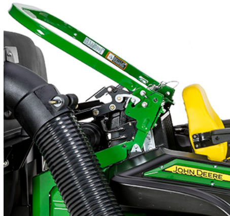
ROPS in intermediate position
