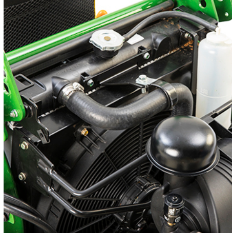
Radiator and electric cooling fan
