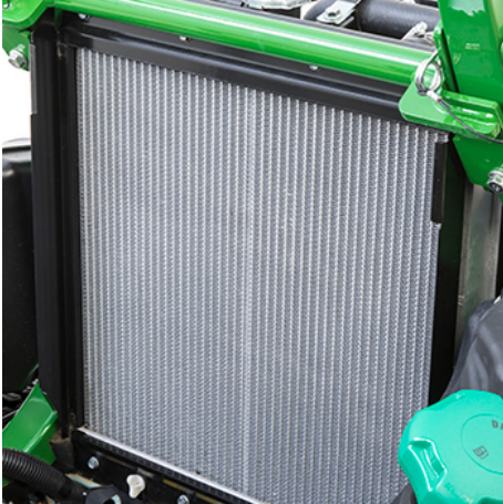
Radiator shown with debris screen removed
