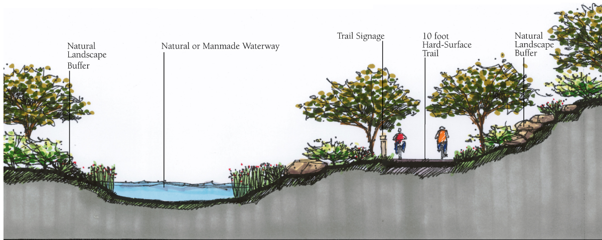
Figure 4.1.2. Typical Hard-Surface Park Trail Cross-Section
