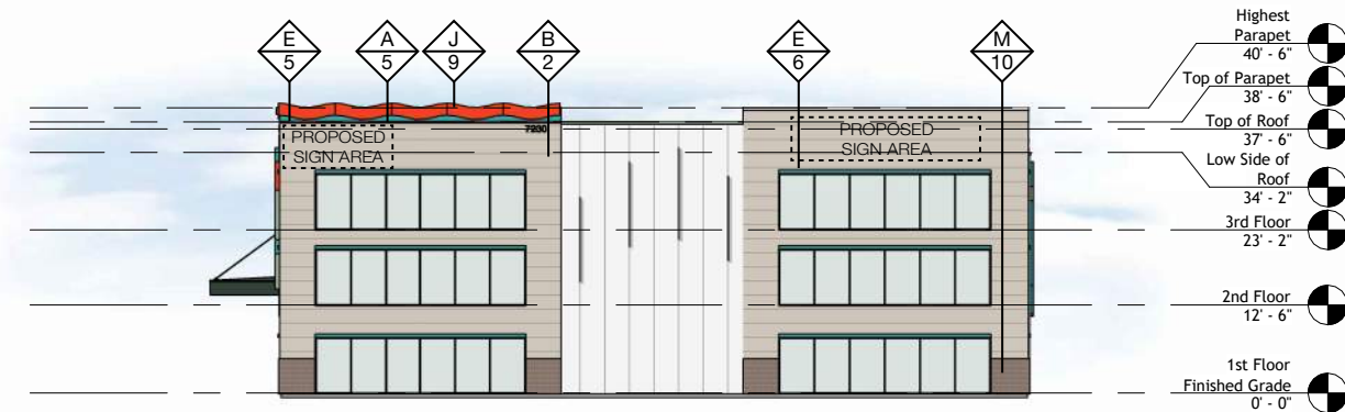
SOUTH ELEVATION - BLDG. A
