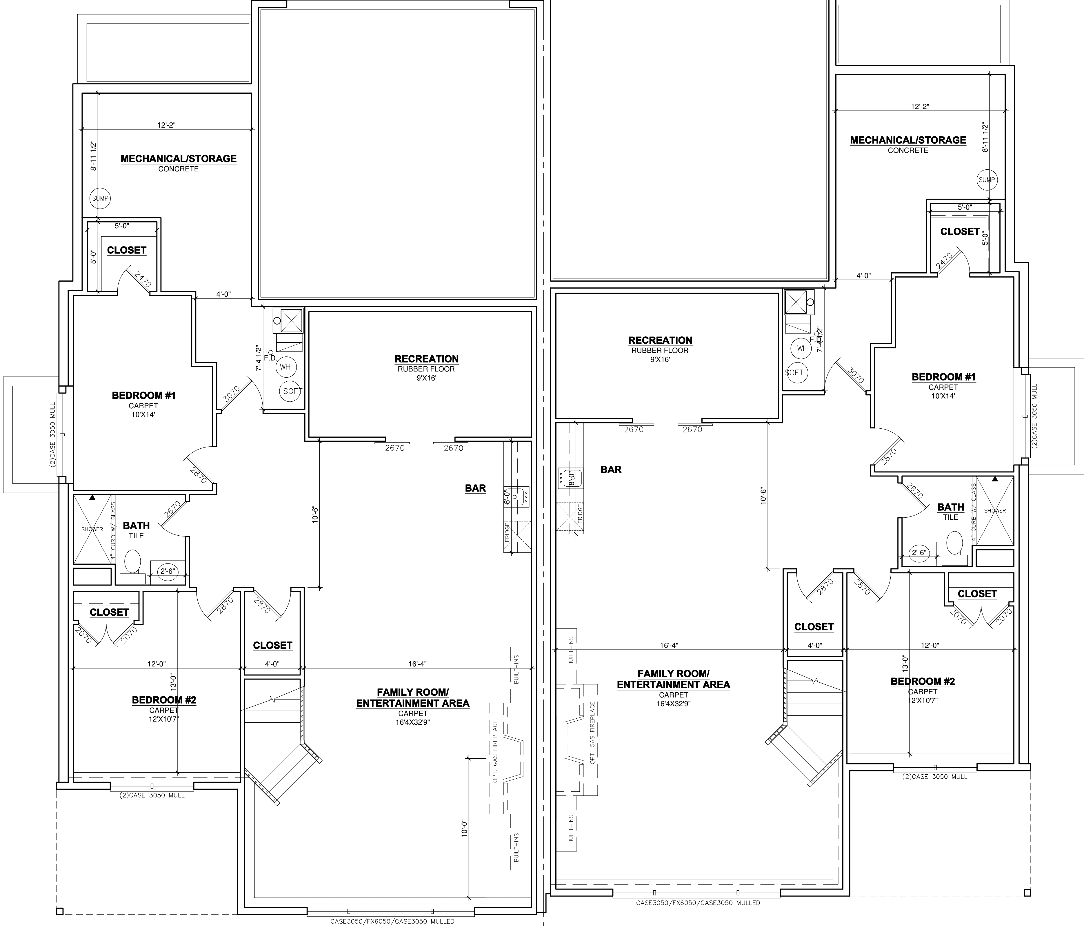
2 PROPOSED UNIT BASEMENT PLAN 1348 FINISHED SQUARE FEET PER UNIT / 200 UNFINISHED SQUARE FEET PER UNIT/ 1548 TOTAL SQUARE FEET (PER UNIT)
