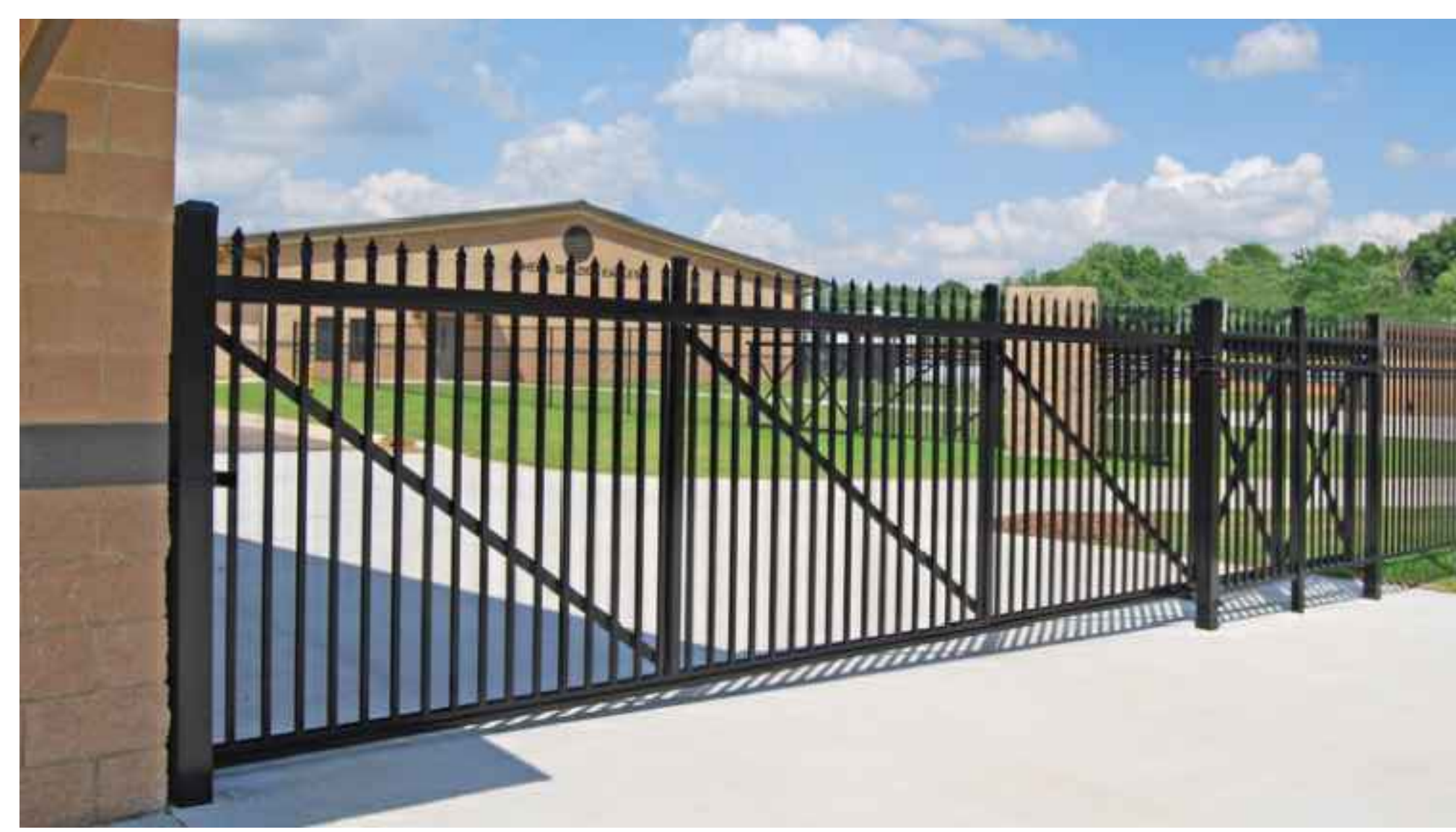
24'-0" x 8'-0" SLIDING ORNAMENTAL GATE FRAMES TO BE MADE OF VERTICAL AND DIAGONAL 2" SQUARE ALUMINUM TUBING x 1/8" THICKNESS. POSTS TO BE MADE OF 4" SCHEDULE 40 GALVANIZED x .125 THICKNESS WITH A MINIMUM STRENGTH OF 35,000 PSI. TRUCK ASSEMBLIES CONSIST OF TWO HEAVY-DUTY SWIVEL TRUCKS ON FOUR HORIZONTAL WHEELS WITH FACTORY SEALED AND LUBRICATED BEARINGS AND TWO HIGH-IMPACT LATERAL WHEELS FOR PROPER ALIGNMENT OF THE TRUCK WITHIN THE TOP TRACK. TOP TRACKS CONCEAL TRUCK ASSEMBLIES FOR PROTECTION AGAINST THE ELEMENTS.
