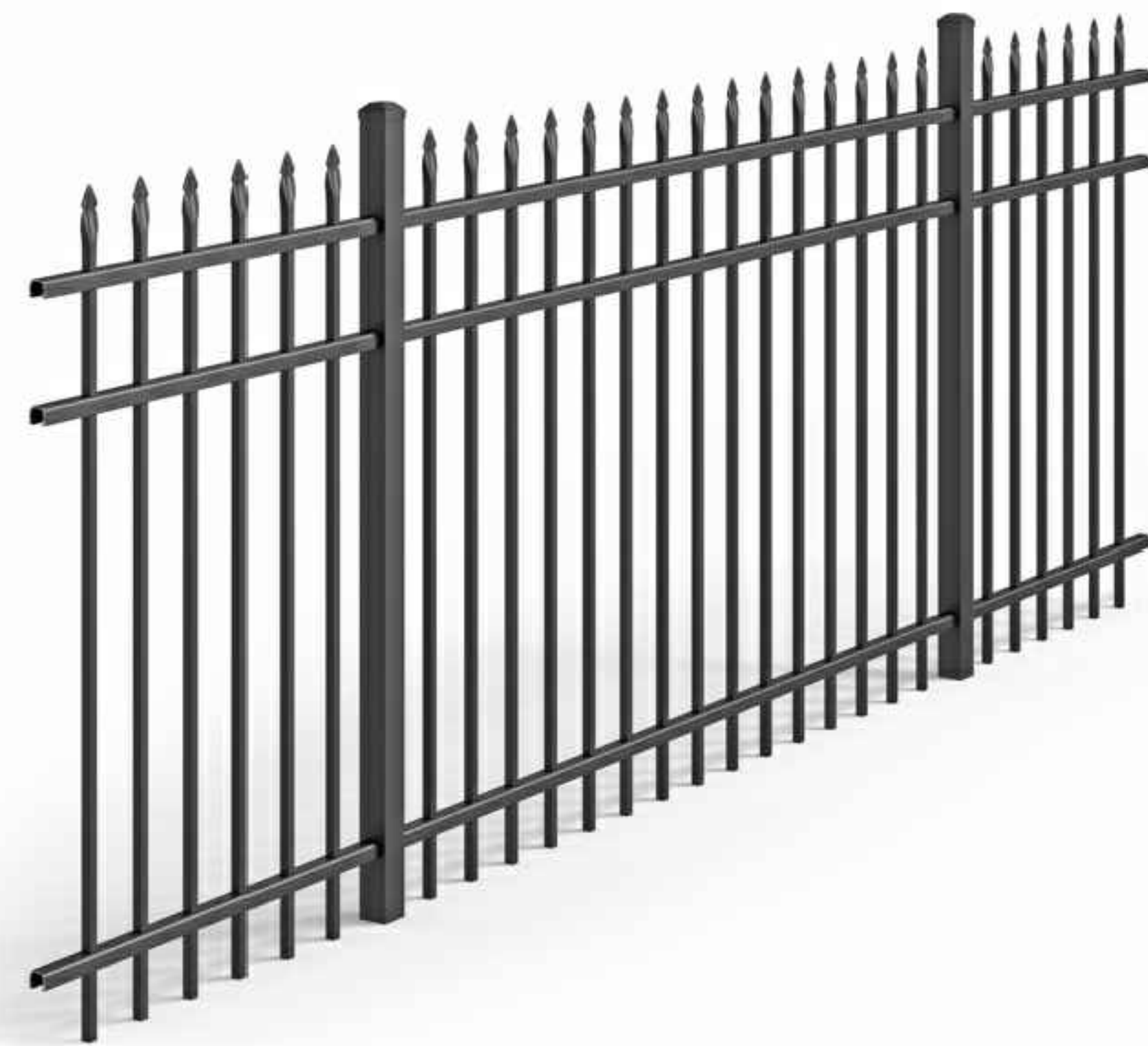
8'-0" ORNAMENTAL IRON FENCE UAS-100 SPEAR TOP FENCE PICKETS TO BE 1" SQUARE x .062 WALL WITH A SPACING STANDARD OF 4" OR THE OPTIONAL 1-1/2". FASTENERS TO BE MADE OF STAINLESS STEEL. HORIZONTAL RAILS TO BE 1-5/8" x 1-5/8" WITH .100 SIDE WALLS AND .070 TOP WALLS. POSTS TO BE 2-1/2" SQUARE x .100 WALL; 3" SQUARE x .125 WALL AND STANDARDS CAPS INCLUDED. FENCE TO BE MADE OF ALLOY WITH MINIMUM STRENGTH OF 35,000 PSI.
