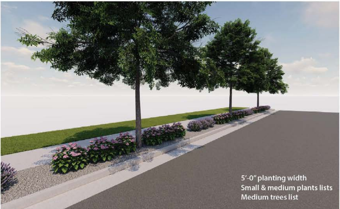
Figure 5.16 - Refurbished park strip example: 5'-0" planting width
