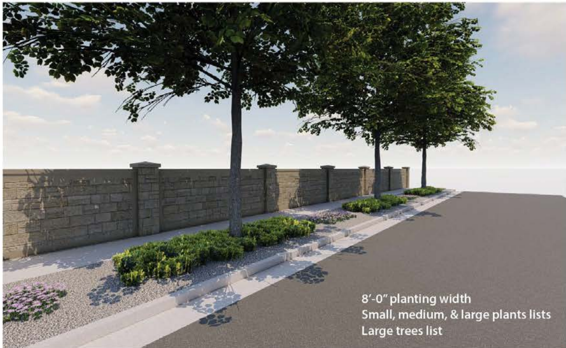
Figure 5.17 - Refurbished park strip example: 8'-0" planting width
