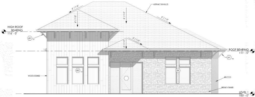
1 SOUTH ELEVATION ELEVATION 1/8" = 1'-0"
