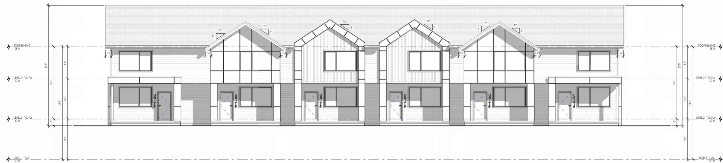
FRONT ELEVATION SD 3/16" = 1'-0"
