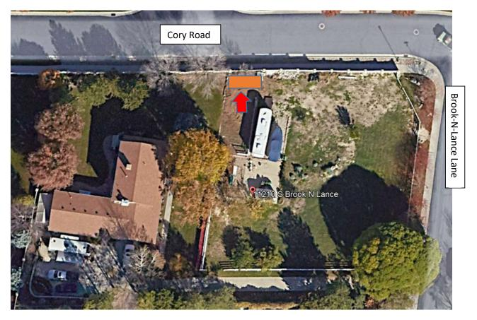
Request for installation of 18'X10' TuffShed (7' Height). As indicated, aligned with North fence about midway. 5' setback.
