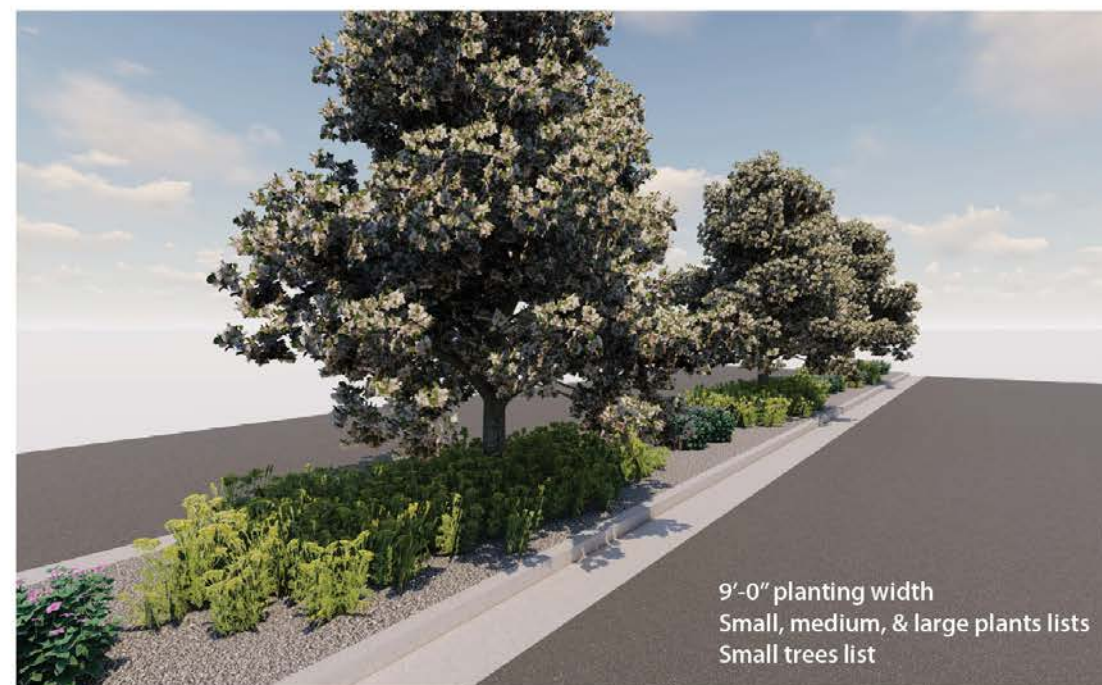
Figure 5.18 - Refurbished median example: 9'-0" planting width of standard 14'-0" median
