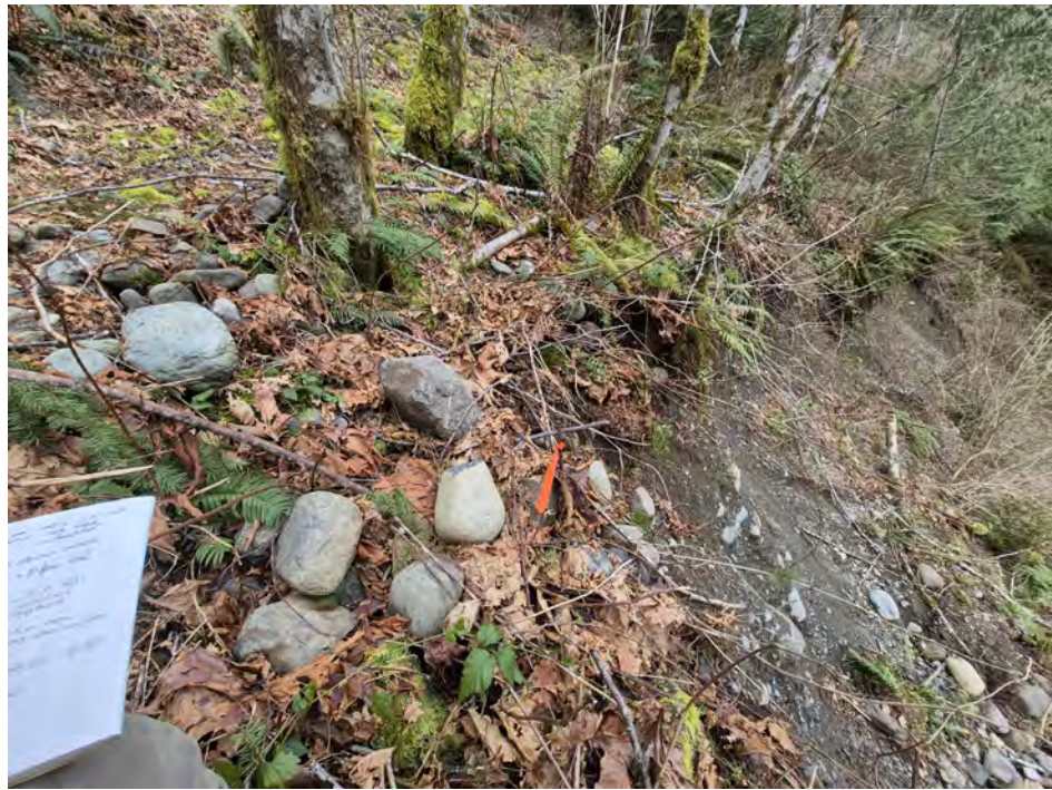
PHOTO 4: Landslide headscarp downslope of the pipeline. Orange flag is AMP-04, STA 41+80. Pipeline is in upper part of photograh, about 11 feet from head scarp.
