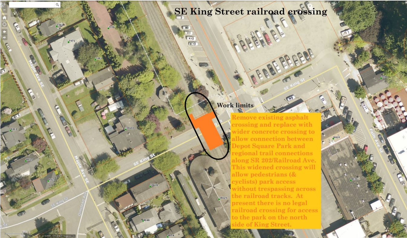
Proposed project work. This is a crossing replacement project to provide a safe and legal crossing from connections with the regional trail network to the city park called the Depot Square Park.
