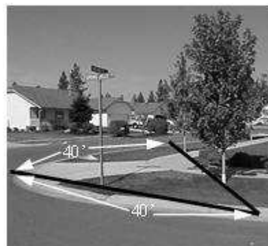
Figure 8: Vision clearance. A vision clearance triangle is 40' from the intersection's road or curb edge.
