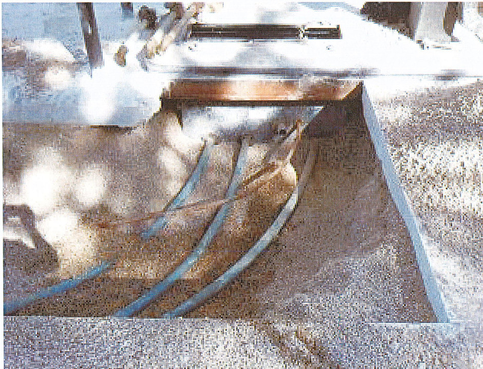
Sample point #1 collected at 3 feet below ground surface beneath the supply lines.
