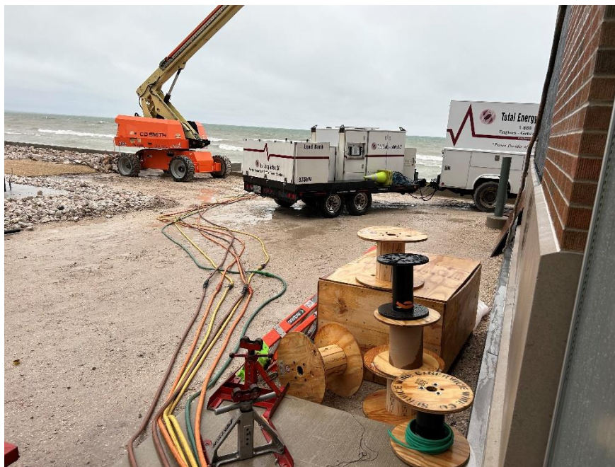
Load bank set up for generator testing.
