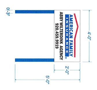
DESC. DIGITALLY PRINTED VINYL, UV LAMINATION, APPLIED TO 3MM ACM PANELS INSTALLED WITH 2-3" POLES, PAINTED CORPORATE BLUE PMS 293C
