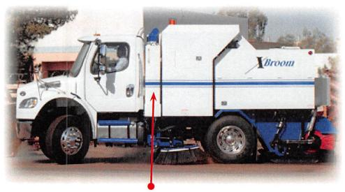
The 40 gallon hydraulic tank is mounted directly behind the cab, high on the left side. This keeps the tank away from the dirt and provides better suction flow to the pumps. There is a large in-tank return filter, glass sight level with a thermometer, and an in-tank float and over-temperature switch for operator warning indicators. Every hose has a female JIC swivel on both ends, making replacement, if necessary, easier.
