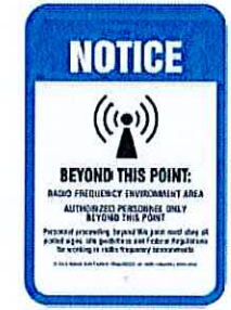
1 NOTICE RF SIGN (BLUE) WHITE/BLUE BACKGROUND, WHITE/BLACK LETTERING MOUNTING LOCATION: GATE & CENTERLINE OF FENCING AROUND SITE (QTY: 4) WHERE ACCESS GATE INSTALLED (QTY: 5)
