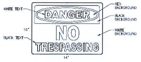
DANGER NO TRESPASSING SIGN WHITE/BLACK BACKGROUND, BLACK/WHITE LETTERING MOUNTING LOCATION: GATE & BASE OF TOWER QUANTITY: 1 WHERE ACCESS GATE INSTALLED (QTY: 2)
