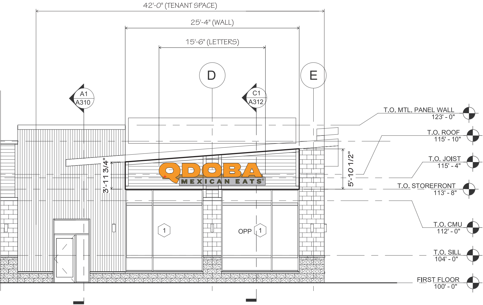
1 SOUTH ELEV. - RACEWAY CHANNEL LETTERS P_02 (1) REQ'D 1/8" = 1' - 0" SCALE
