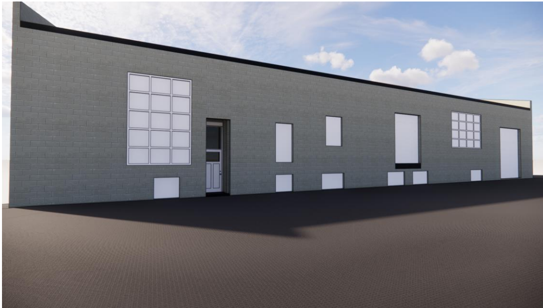
Proposed New southwest Elevation showing storefront glazing in existing openings.
