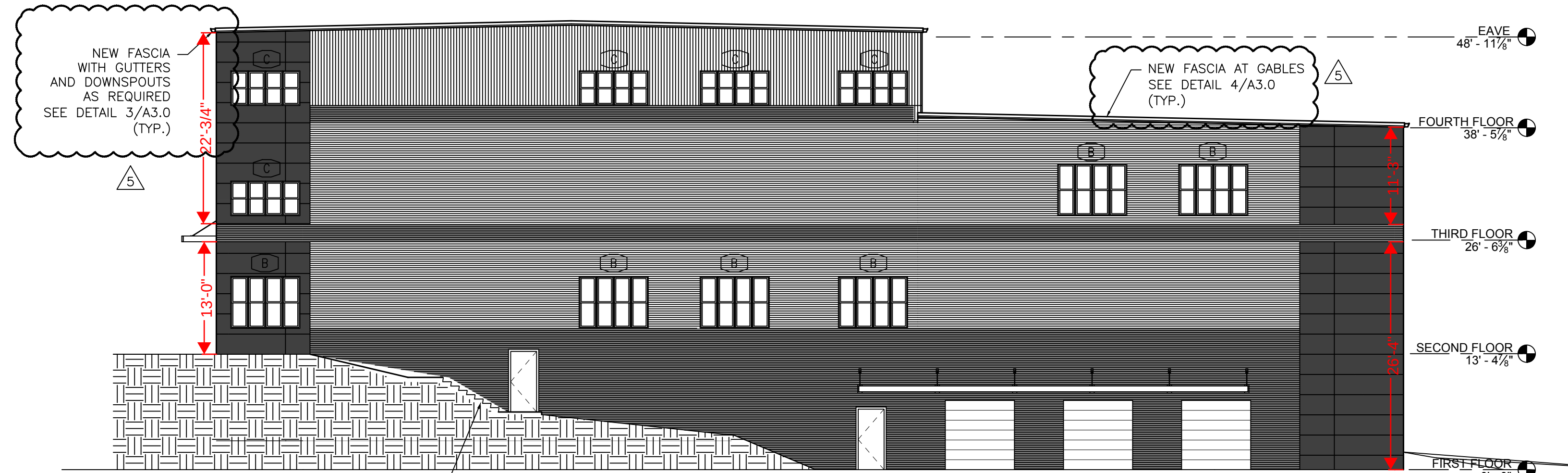
EAST ELEVATION SCALE: 3/32"=1'-0"
