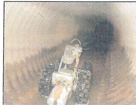
Typical CCTV Camera in Pipe
