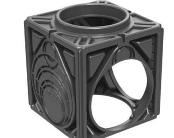
If using more than one access chamber module in a stack, it will be necessary to remove base from all modules except bottom base unit. Cut along the recessed cutting line provided and remove base.
